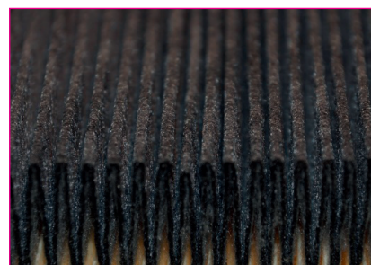
Fig. 1: Activated charcoal filter media pleated (source: Jowat)
