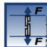
When determining the heat resistance in accordance with the testing standard DIN EN 14257 (Watt 91), tensile shear strengths of > 10 N/mm<sup>2</sup> are achieved at 80° Celsius. Values of > 7 N/mm<sup>2</sup> would already be sufficient to meet the recommendation for the manufacture of window scantlings. Several adhesive systems also considerably exceed the tensile shear strengths required for durability class D4 (according to DIN EN 204/205).
